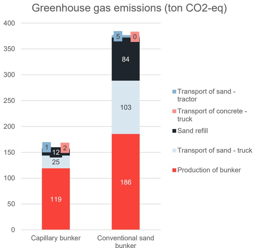
Figure 1 Greenhouse gas emissions from capillary concrete golf bunkers and conventional golf bunkers at an 18-hole golf course over 25 years
